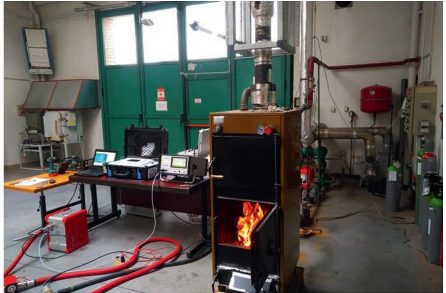
Figure 6: Laboratory examination of combustion equipment
